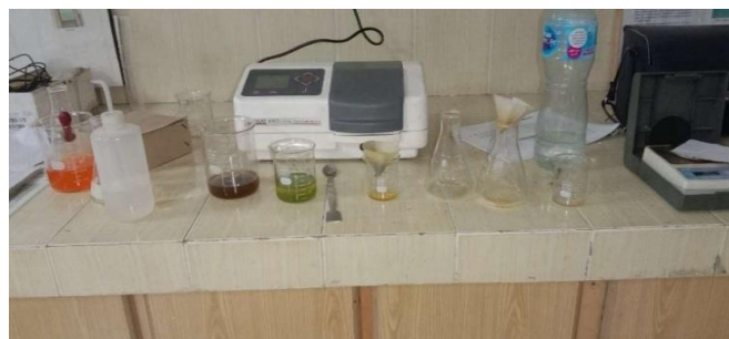
Figure 9: Spectrometer with some mixture of coagulants and wastewater
